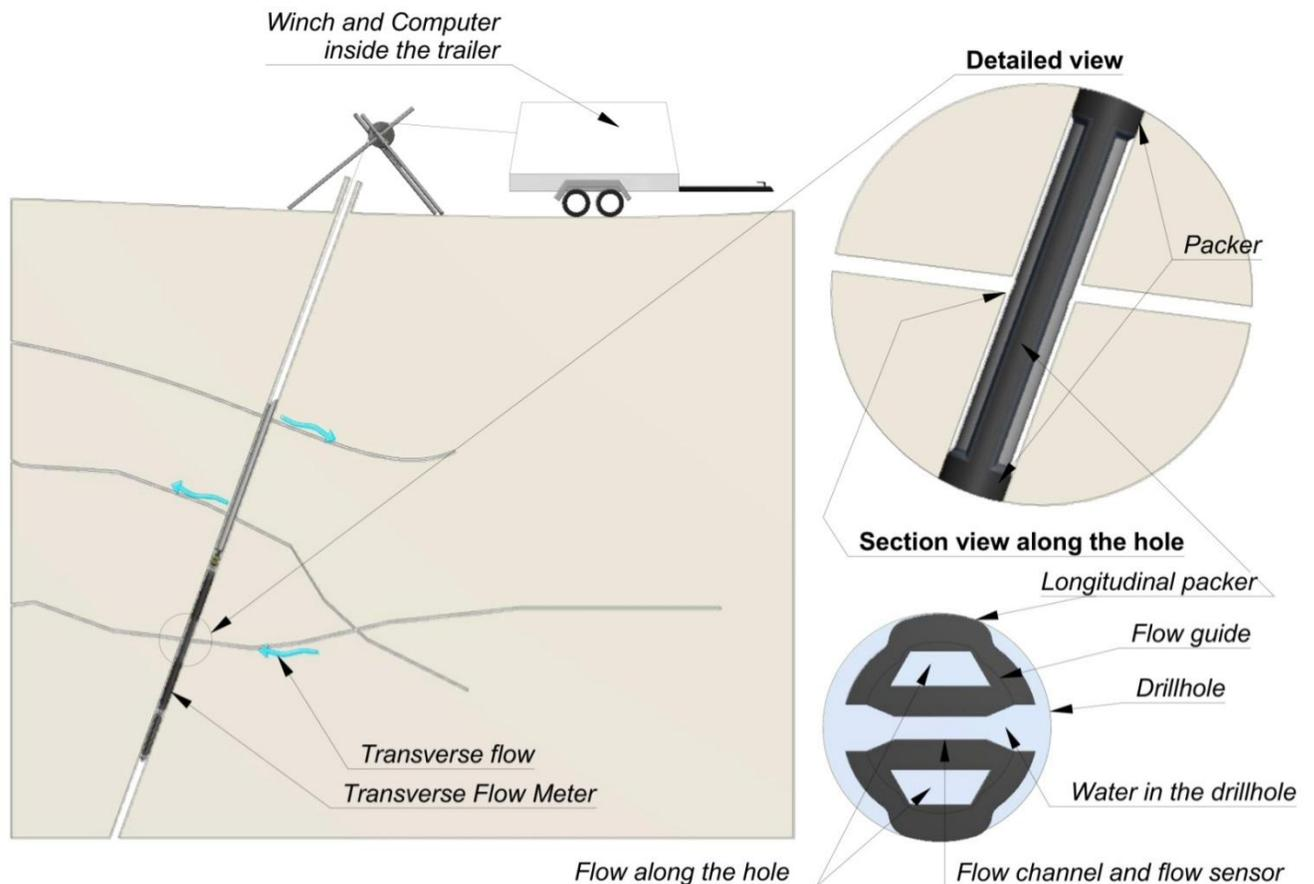
**Figure 1.** Schematic of the probe used in the PFL TRANS.
