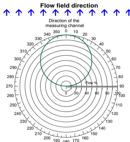
**Figure 3.** Flow pattern with different probe orientations.
